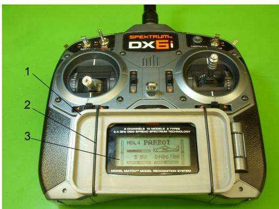
Fig. 18. Clamp on Transmitter
